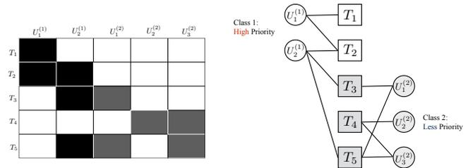
Fig. 1. Spatially coupled-based networks with prioritization: (a) An example of random access table describing the accesses of two classes  $U_i^{(1)}$  and  $U_i^{(2)}$ , where users of Class 1 have access to all time-slots, while users of Class 2 have only access to time-slots  $T_2 - T_5$ , and (b) A bipartite graph representing a wireless network having two classes with high and less priority.
