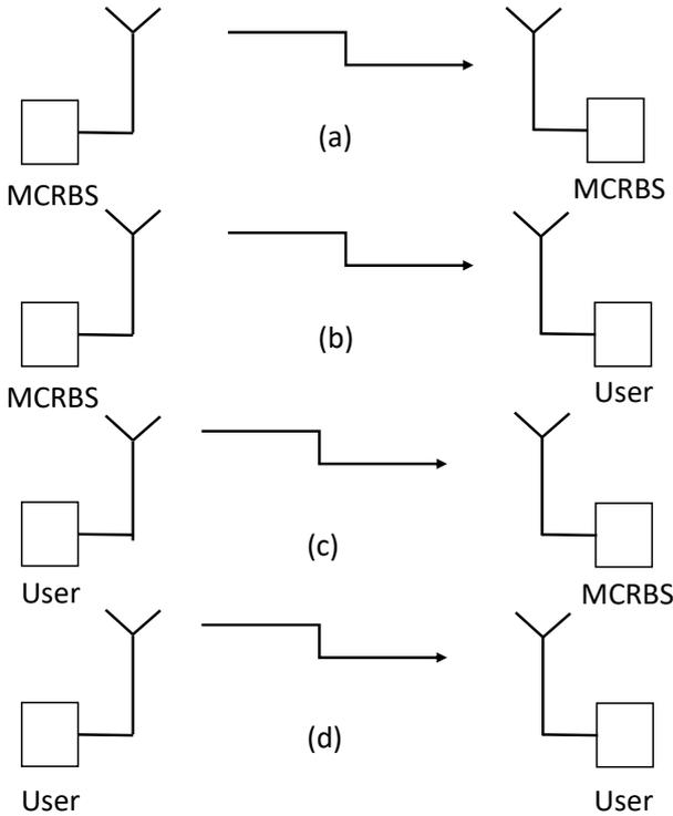
Fig. 2. Type of link models: (a) communication link from MCRBS to MCRBS, (b) communication link from MCRBS to user, (c) communication link from user to MCRBS, and (d) communication link from user to user.
